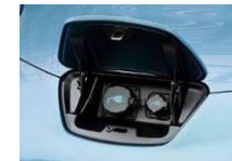
EV Charger outlet
